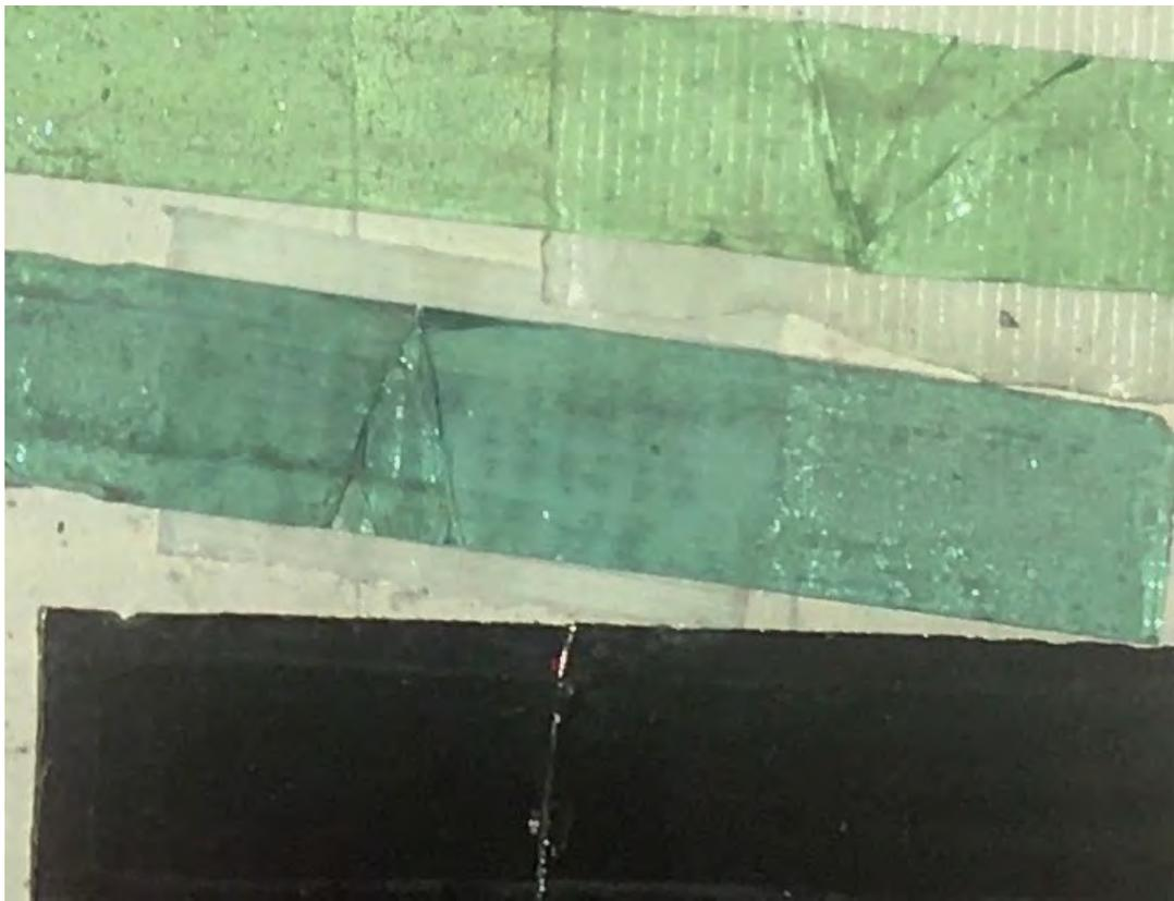
*Figure 24: Variety of stress cracks from an unknown cause, from glass at the edges of a panel.
