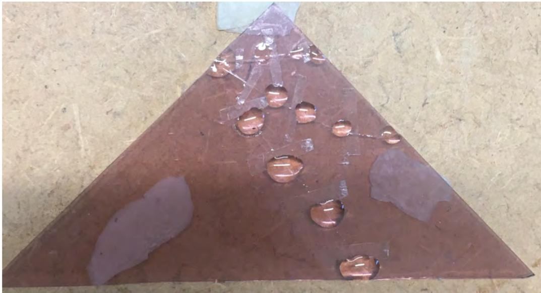
*Figure 55: Piece for the panel after the drops of adhesive were placed on the fractures. The fractures were caused by a stress of glass pliers on the edge of the glass. Image by L.Ristal, 2022.*
