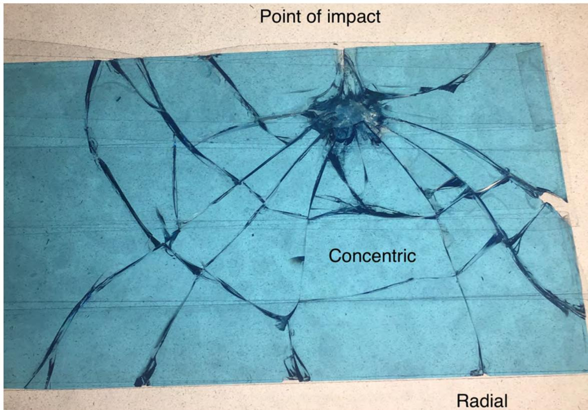
Figure 27: Impact crack caused by a stone throw to the piece of glass that was on the floor. Image by L.Ristal, 2021.
