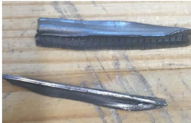
Figure 46: The lead came with one of the top parts separated.
