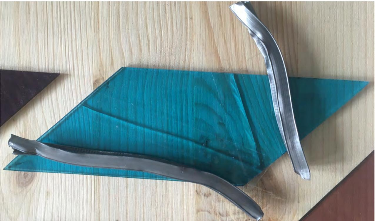
*Figure 40: The glass with the lead came roughly cut. Image by L. Ristal, 2022.*
