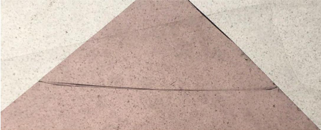
*Figure 23: Stress crack made by making a small crack and applying pressure with glass pliers.
