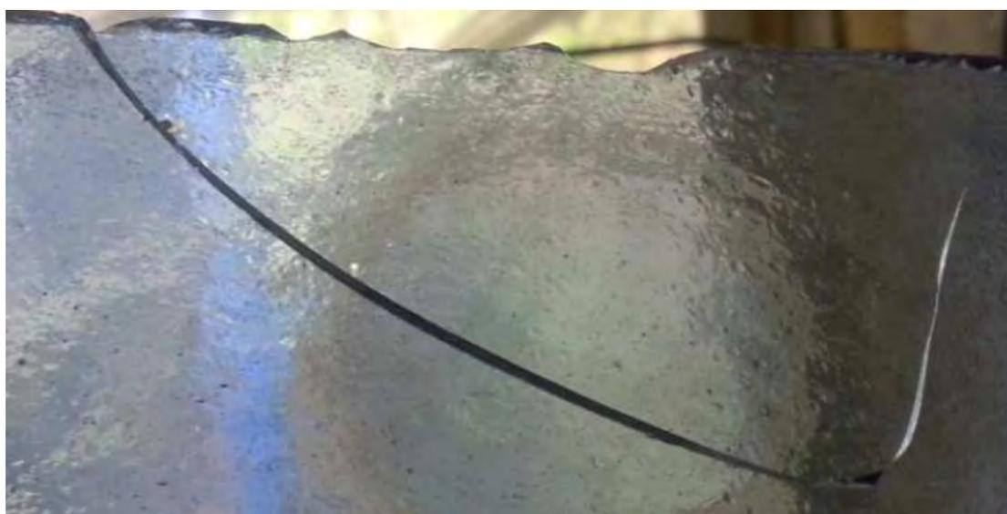
Figure 25: An incomplete crack. Image by Sean Hardigan, May 2013, from *An Analysis of Stained Glass Fabric Specific to Conservation Assessment*, p 8.
