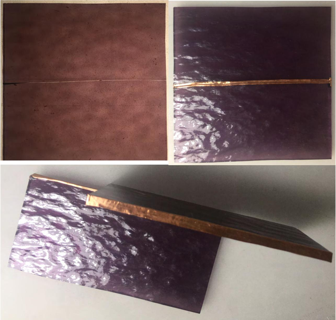
*Figure 49: The crack and copper foiled edges from the side and top point of view. Image by L.Ristal, 2022.*
