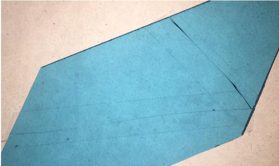
*Figure 39: The piece from the panel that will be re-lead. The damage is a stress crack from dropping the piece and adding pressure with glass cutting pliers. Image by L.Ristal, 2022.*
