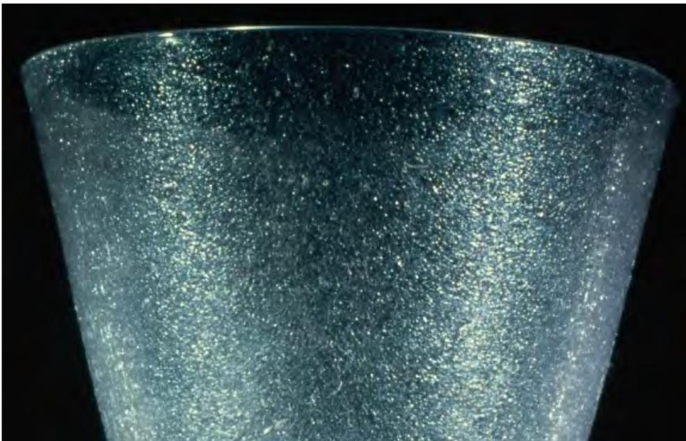
*Figure 22: Uniform cracking of the surface of a goblet, illustrating the third stage of crizzling (full-blown crizzling). Image by Corning Museum of Glass, from article Crizzling, All About Glass, Corning Museum of Glass, 08.XII 2011, <https://www.cmog.org/article/crizzling> (Accessed 02.V 2022).*
