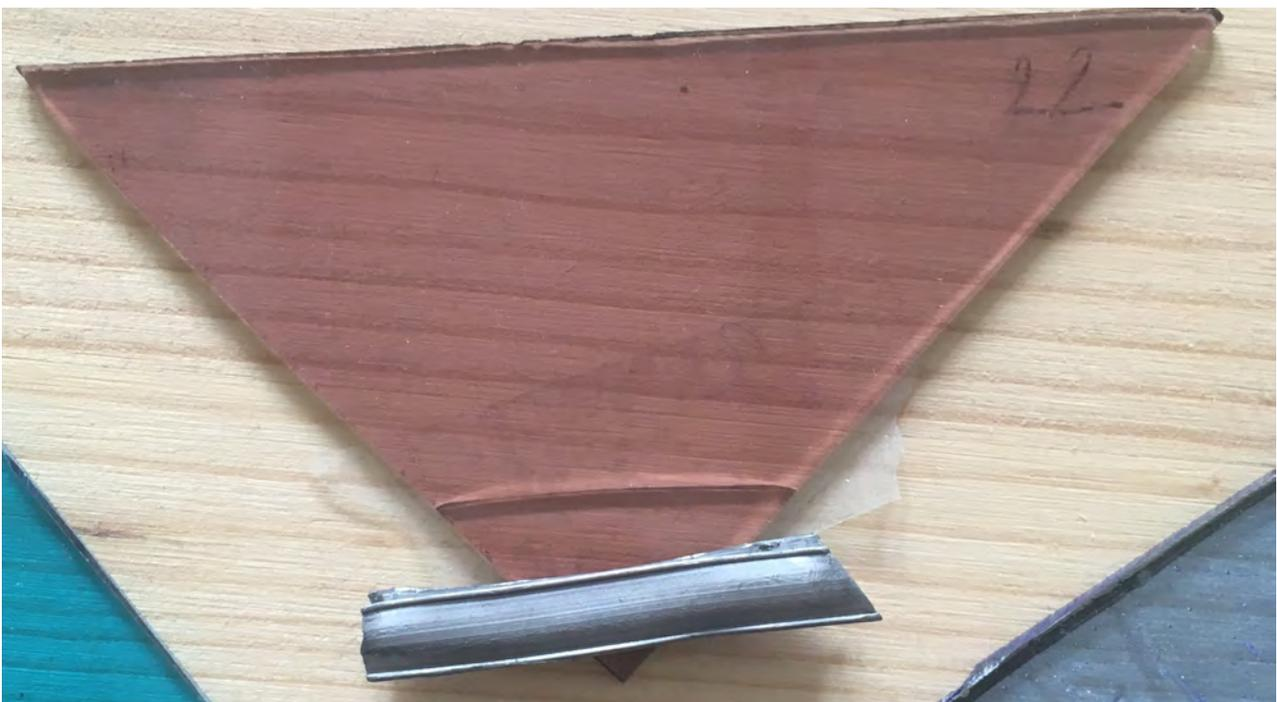
Figure 44: The glass with the lead came roughly cut to size of the crack. Image by L. Ristal, 2022.
