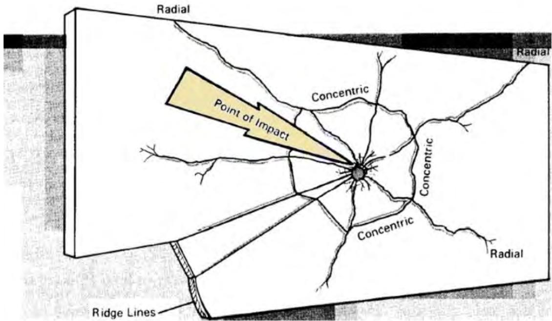
Figure 26: Figure Showing Radial And Concentric Cracks Upon Impact. Image from V. D. Crawford, *Glass Analysis: Types Of Glass, How To Determine The Density Of Glass, And Analysis Of Glass Fracture Patterns*, 2014, p 4.
