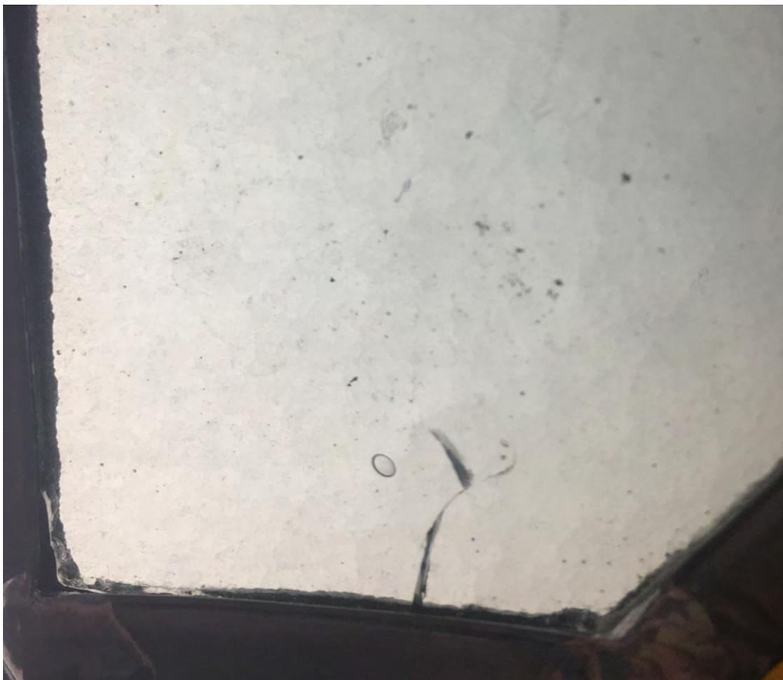
*Figure 29: Incomplete heat crack caused by the tip of the soldering iron on glass. Image by L.Ristal, 2021.*
