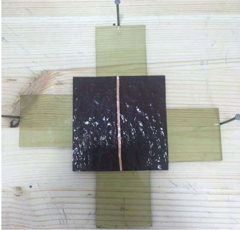
*Figure 50: The two pieces secured in place with four pieces of glass. Image by L.Ristal, 2022.*
