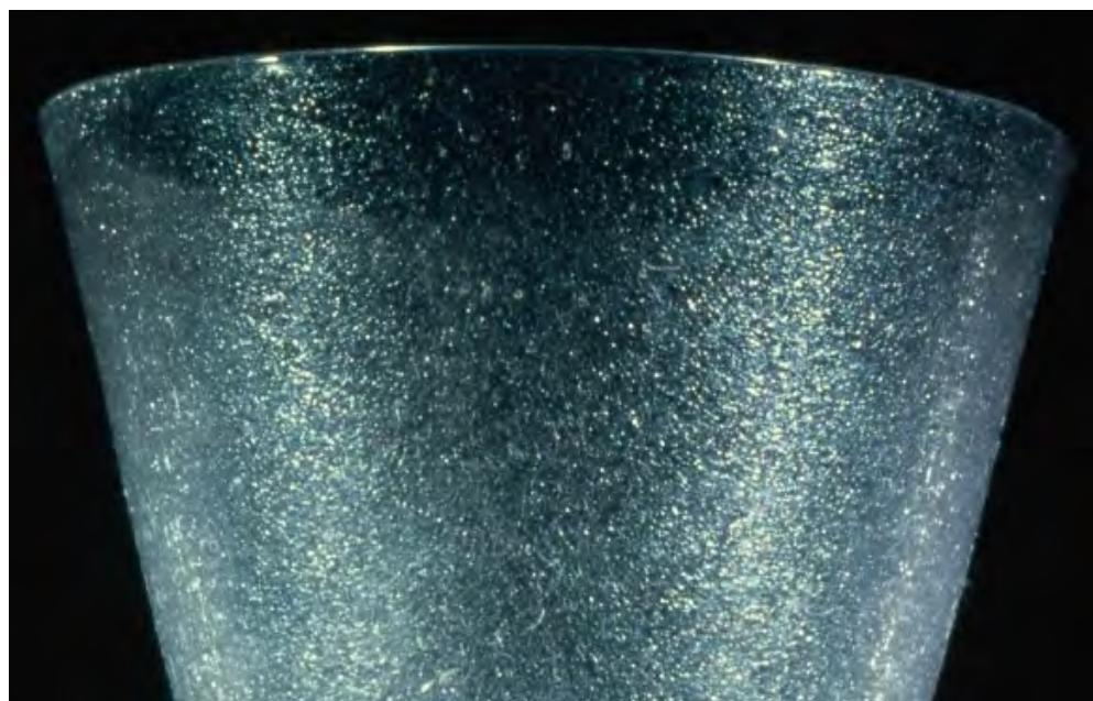
Figure 22: Uniform cracking of the surface of a goblet, illustrating the third stage of crizzling(full-blown crizzling). Image by Corning Museum of Glass, from article Crizzling, All About Glass, Corning Musem of Glass, 08.XII 2011, <https://www.cmog.org/article/crizzling> (Accessed 02.V 2022).
