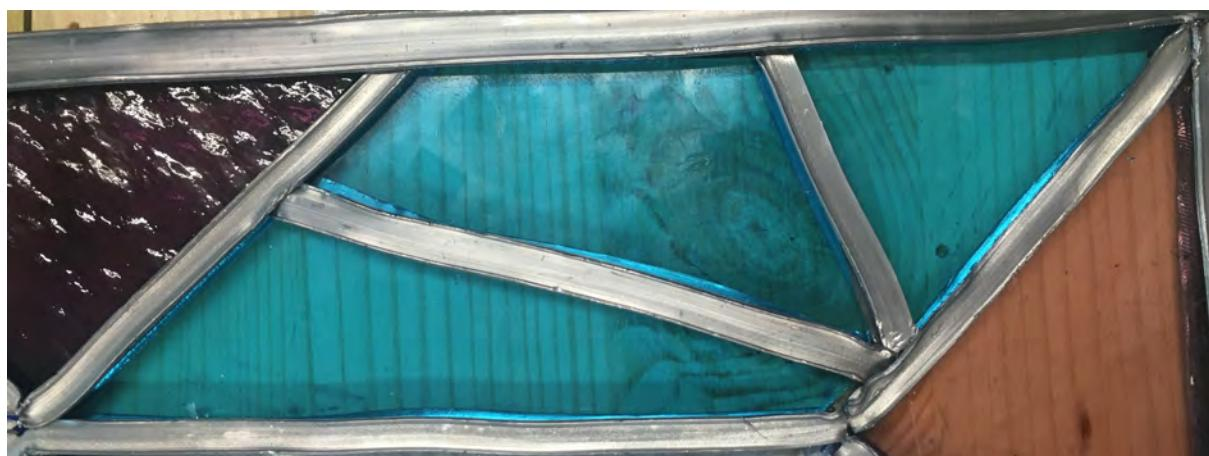
Figure 42: The piece with the lead came inserted into the panel, unsoldered. Image by L.Ristal, 2022.
