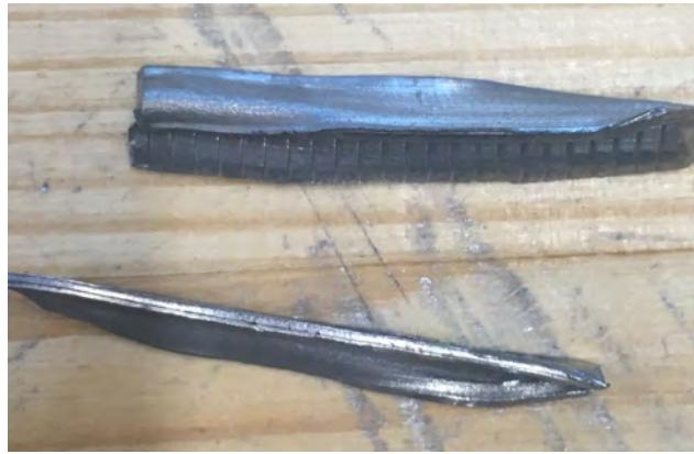
*Figure 46: The lead came with one of the top parts separated.*
