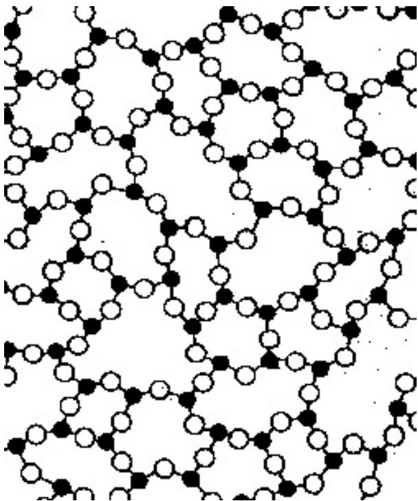
*Figure 20: The molecular arrangement in a fused silica glass.*
