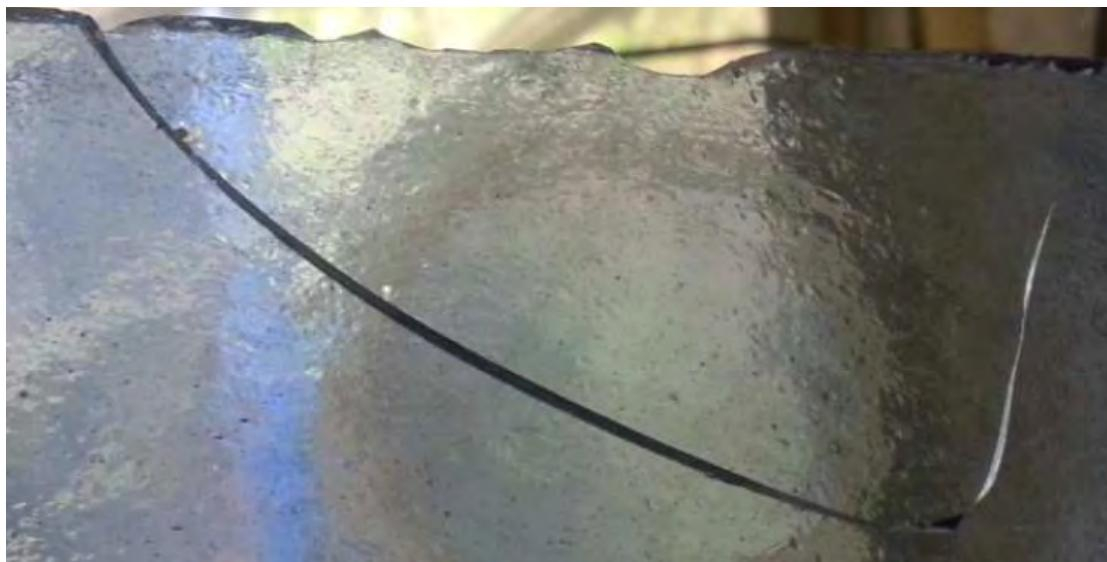
Figure 25: An incomplete crack. Image by Sean Hardigan, May 2013, from *An Analysis of Stained Glass Fabric Specific to Conservation Assessment*, p 8.
