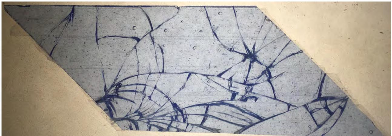
Figure 34: Picture of a severely impact damaged piece that had to be replaced. The piece was damaged by a chair falling onto it, as can be seen from the multiple impact points. Image by L.Ristal, 2022.
