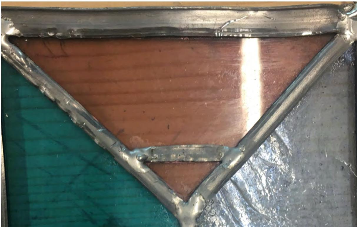
Figure 48: False lead soldered into place on the crack. Image by L.Ristal, 2022.
