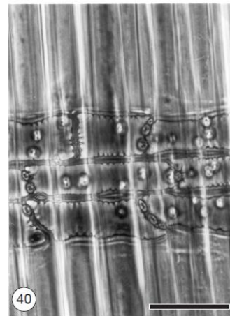
Fig. 40. Cell walls of ray tracheids, radial sections. Cell walls with helical thickenings resembling fine dentations (feature 69). Picea abies .
