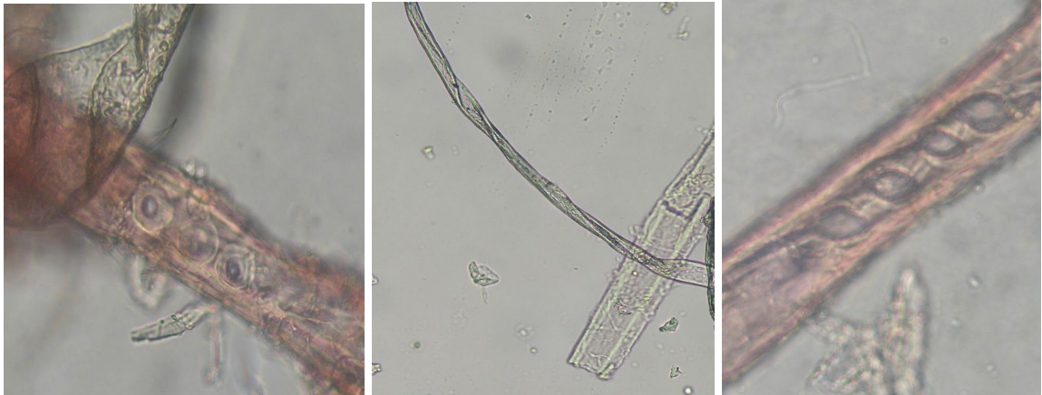
2.23. Left: round coniferous tracheids; middle: long fibre of cotton and fibre of linen; right: square deciduous tracheids.
