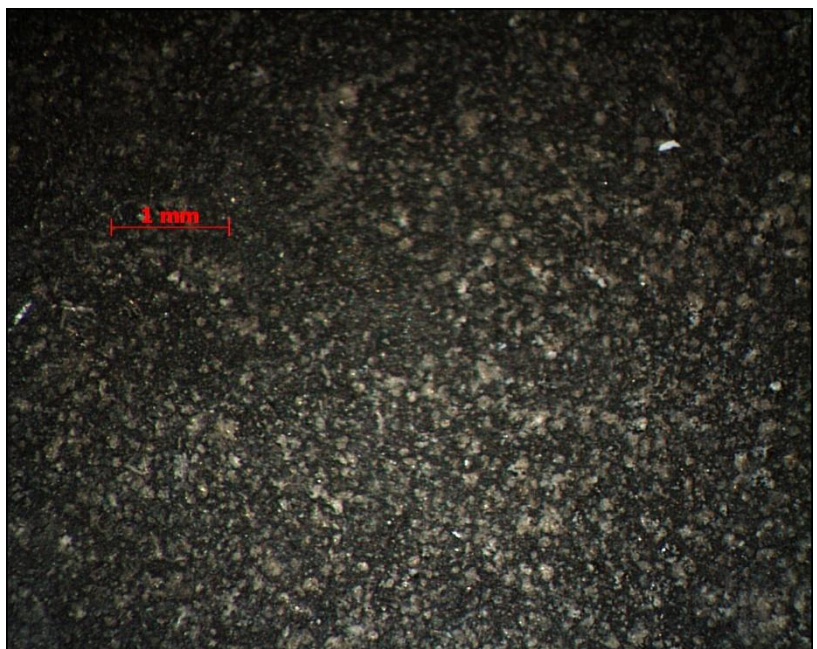
Figure 13. Closely placed pit corrosion that in transmitted light fog up the glass. 2,5x magnification.
