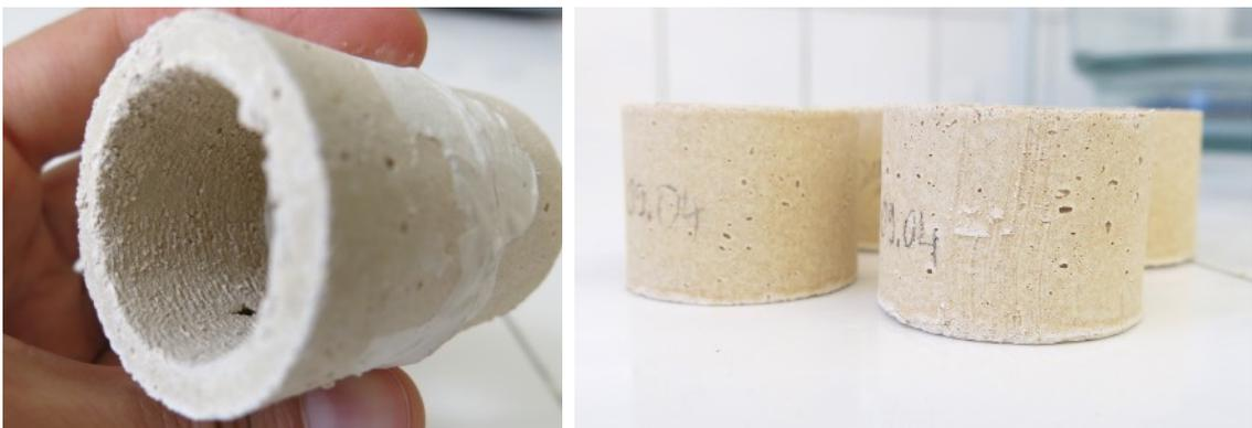
3. Two cylinders were glued together with the mixture of NHL 5 and water (see ill. 37).
