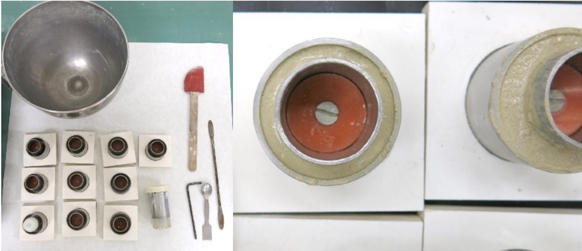
2. The inner surface of the specimen was coarsened before it was taken out of the cast, and left to cure for 28 days. The dimensions of the specimens were 40x40x5 mm (see ill. 36).
