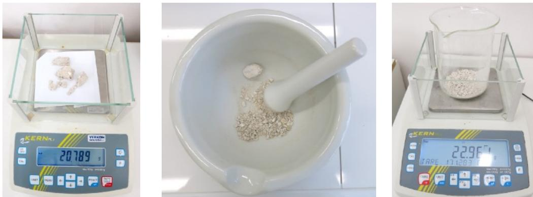
3. The crushed samples were put into a 600 ml glass container and weighed again.
