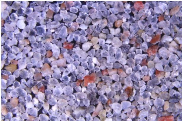
20. TV-W-1. Fraction of the sand is 0,25mm. Magnification: x10.
