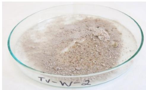
8. To calculate the percentage of the sand the total weight of the sand (2<sup>nd</sup> weight) was subtracted from the weight of the crushed sample (1<sup>st</sup> weight) and the result was multiplied with 100. The percentage of dissolved binder is equal with the percentage of the sand subtracted from the 100%.<sup>42</sup>
