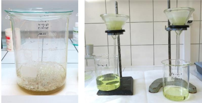
6. After filtering, the filter paper together with the sand was placed on a petri dish and dried in the oven at 45°C for two hours.
