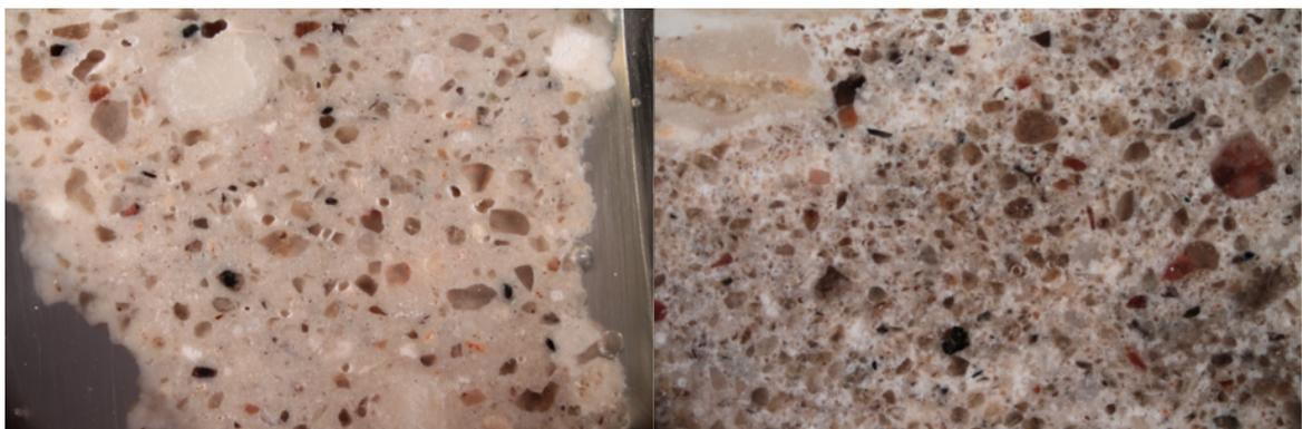
Fine particles of quartz (transparent/white) and granite (light red) sand can be seen in these optical microscope photographs, taken from the sand of both samples, TV-V-1 and TV-W-1 (see ill. 19 and 20).
