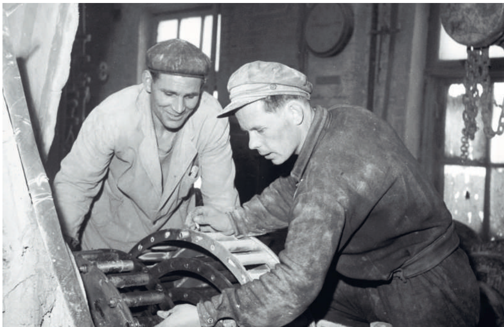
4.04: Männiku Ehitusmaterjalide Tehase töölised desintegraatori korvi vahetamas. Workers at the Männiku building material manufacturing plant changing the cage on the disintegrator.
